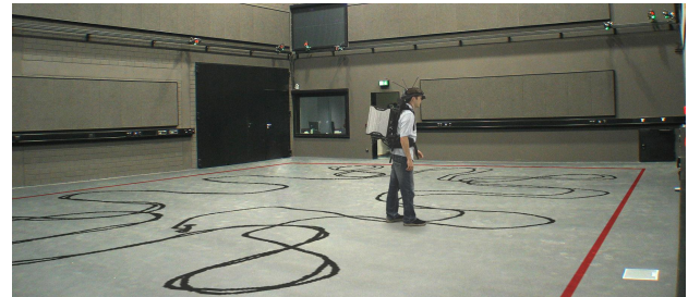
Figure 1: Left: A subject's view along a path through a virtual city. Right: The subject's path bent into a tracked space using our controller.
