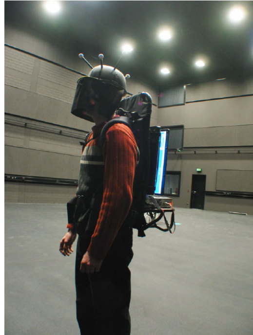
Figure 2: Participant in the Tracking Lab, equipped with tracking helmet, HMD, and notebook computer mounted on a backpack.
